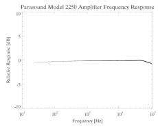
The frequency response of the amp is also flat to about 50 kHz and then very gently rolls off. The rolloff is very small (less than 1 dB) and may be a measurement artifact, as with the preamp measurement. Amplifier crosstalk was not measurable with my measurement setup. The dynamic range of the setup with the voltage divider was insufficient to measure the crosstalk above the noise floor of the measurement setup.
