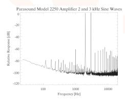
The intermodulation spectrum resulting from 2 kHz and 3 kHz sine waves at the input shows a 1 kHz intermodulation product 60 dB down.
