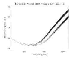
Crosstalk is below the noise floor of the sound card at -85 dB below 1 kHz, and rises to around -60 dB at 20 kHz. The crosstalk
