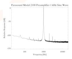
Here we see the output of the preamp with a 1 kHz sine wave at the input. Harmonics are at least 90 dB down from the signal, with the second harmonic the highest in amplitude. The more objectionable third harmonic is more than 10 dB lower in amplitude.
