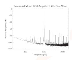
The output of the model 2250 with a 1 kHz sine wave at the input into a 8 ohm power resistor is shown here. Harmonics are at least 60 dB down, with odd harmonics at higher amplitude than the even harmonics. Harmonics are clearly visible to relatively high order (10th harmonic).
