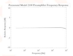
Frequency response is flat as a pancake from 20 Hz to 50 kHz, and rolls off by less than a dB to the Nyquist frequency of the sound card ADC at 96 kHz. These data have been normalized to the frequency response of the sound card.
