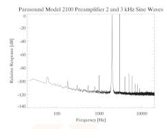
The intermodulation spectrum shows the output of the preamp with 2 and 3 kHz sine waves at the input. The 1 kHz intermodulation product is also about 90 dB down from the signal tones.
