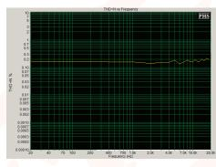
The THD+N vs. Frequency of the 2250 is a low 0.2% from 20 Hz to 20 kHz, and is essentially flat. I also measured THD+N into 4 ohms and 2 ohms and got essentially identical results.
