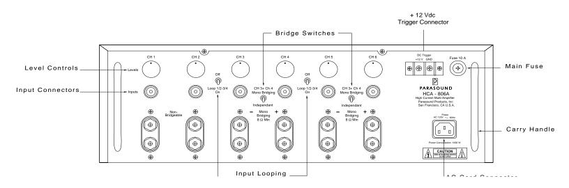
Figure #2 HCA-806A Front Panel Controls
