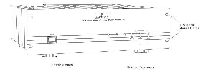
Figure #1 HCA-806A Front Panel Controls
