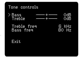
The **Treble tone** control now offers you a choice of three frequencies where the treble tone control range is centered, 6 kHz, 8 kHz and 10 kHz.
